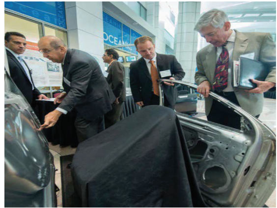
Attendees compare a 40-lb door and a 25-lb aluminum prototype at the American Energy and Manufacturing Competitiveness Summit in September 2014 in Washington, D.C.
